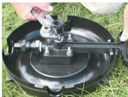
Insert the Hansen Hex Nipple into the Pod Skid Base. Then screw on the Hansen 20mm Female Socket.
