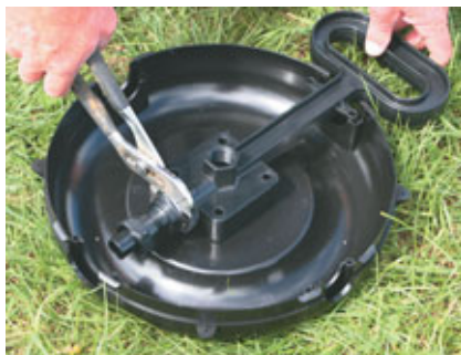
Screw on the Hansen Female Straight Coupler to the end of the handle.
