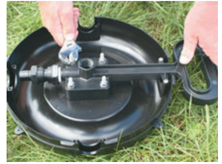
Attach the handle to the Pod Skid with the 4 bolts and screws.
